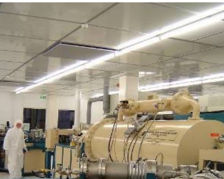
MeV ion accelerator 1 MVolt terminal voltage
