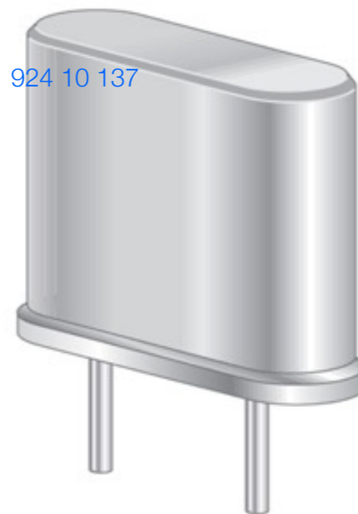
(c) Typical packaged crystal
