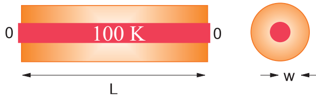
Figure 17.12 A metallic bar insulated along its length with its ends in contact with ice.
