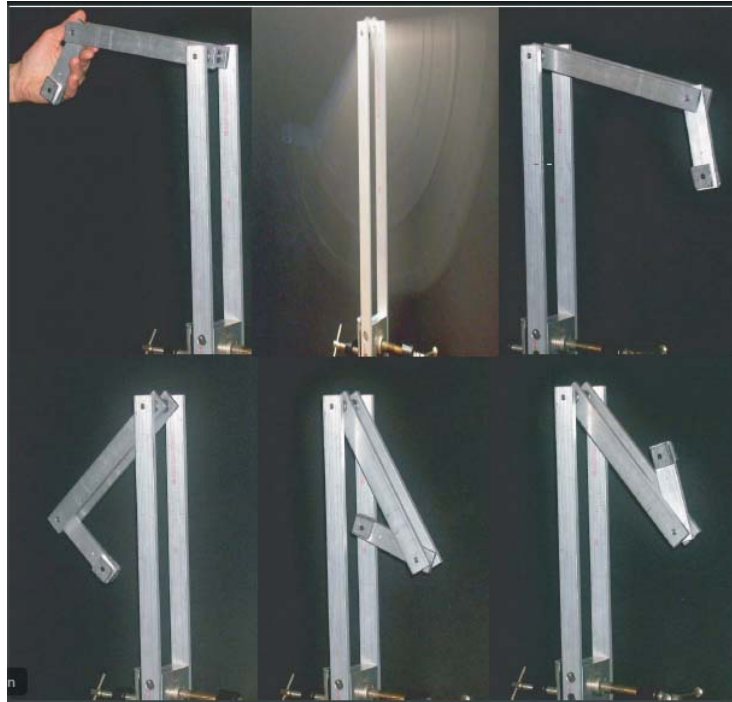
Figure 12.13 Photographs of a double pendulum built by a student in the OSU Physics Department. The longer pendulum consists of two separated shafts so that the shorter one can rotate through it. Both pendula can go over the top. We see the pendulum released from rest and then moving quickly. The flash photography stops the motion in various stages. (Photograph, R. Landau.)
