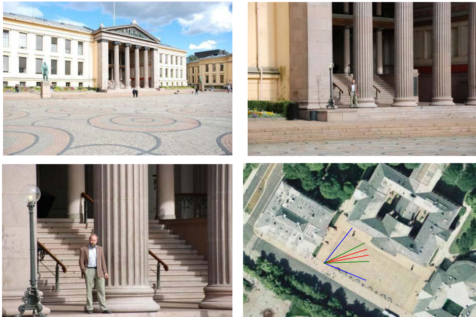
Figure 2-42. Three different images of the same scene using focal lengths f = 18 , 70, and 200 mm. The fields of view of this digital SLR camera illustrated in blue, green and red in the lower right hand aerial image correspond to approximately 1.5 times longer focal lengths in cameras using standard 35 mm photographic film (image area 24 x 36 mm).
