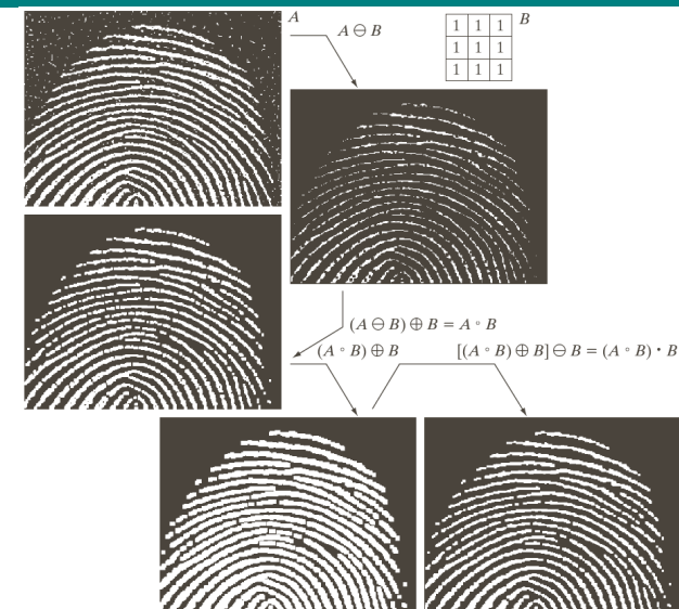
FIGURE 9.11 (a) Noisy image. (b) Structuring element. (c) Eroded image. (d) Opening of A . (e) Dilation of the opening. (f) Closing of the opening. (Original image courtesy of the National Institute of Standards and Technology.)
