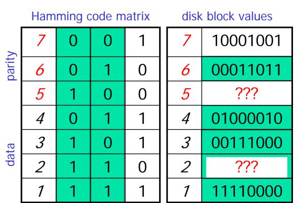
Note 3: restoring disk 2: 11110000 ⊕ 01000010 ⊕ 00011011 = 10101001 Note 4: restoring disk 5 can now be done using column 1
