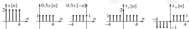
FIGURE E 2.3.b The signal x[n] and its odd and even parts for Example 2.3(b)
