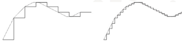
FIGURE 7.29 Staircase reconstruction of a signal at low (left) and high (right) sampling rates. Higher sampling rates produce a much better approximation to the underlying signal and allow the use of a simpler post-filter to smooth out the edges
