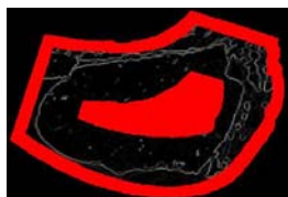
Find internal and external markers from gradient image
