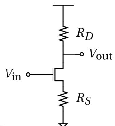
$$G_m = \frac{g_m}{1 + g_m R_S} \approx \frac{1}{R_S}, \quad g_m R_s \gg 1$$
