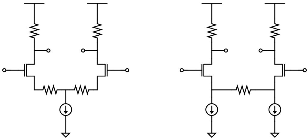
Resistive degeneration also works for diff pairs
