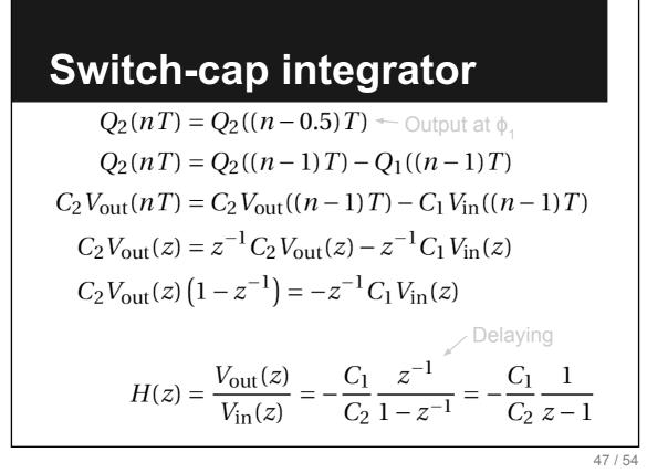
Switch-cap integrator Approx frequency response:  $z = e^{j\omega T} \approx 1 + j\omega T$ Valid when  $\omega T$  is close to zero. I.e. when signal frequency is low compared to sampling freq.  $H(z) = -\frac{C_1}{C_2} \frac{1}{z-1}$ Compare to continuous time  $H(e^{j\omega T}) \approx -\frac{C_1}{C_2} \frac{1}{j\omega T}, \quad \tau = T\frac{C_2}{C_1}$
