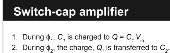
If  $C_1$  and  $C_2$  are of different value, the same charge will give a different voltage drop
