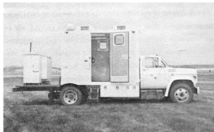
"Mobile" Wireless Sensor Node. DSN test bed around 1985
