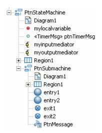
StateMachines used as submachines can have entry/exit points, but make sure to add any entry/exit point to the statemachine and not the region.
