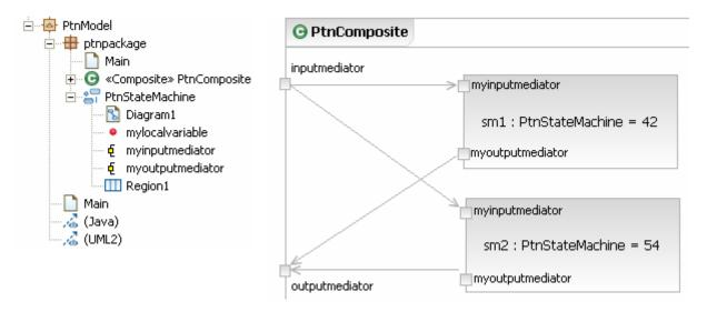
In the figure above PtnComposite has two parts, both of type PtnStateMachine. PtnStateMachine has a parameter called mylocalvariable of type int. The figure below shows sm2's Default Value field set to 54.
