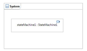
When adding a **Part** to a **Composite structure** selecting a StateMachine under "Select an existing element" is not possible. There are two ways to do this:
