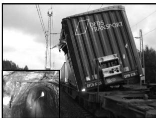
The lateral safety mechanism not attached before departure, causing a blow to the container to tilt it out of position and causing further damage to the track material along the way
