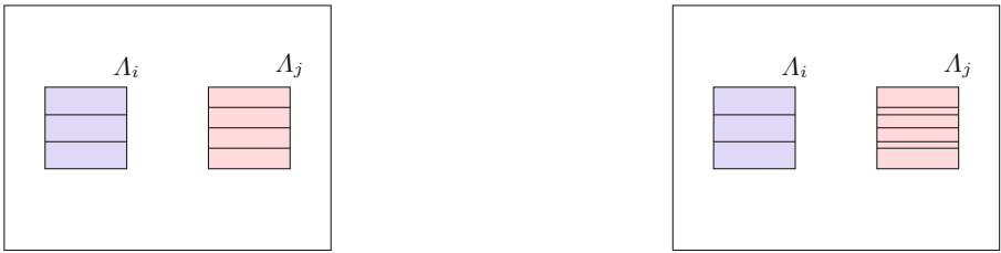
Fig. 4. Left: TBPN-splines allow to refine the subdomains A_a and A_b independently. Right: THB-splines require nested knot vectors for any pair of subdomains.
