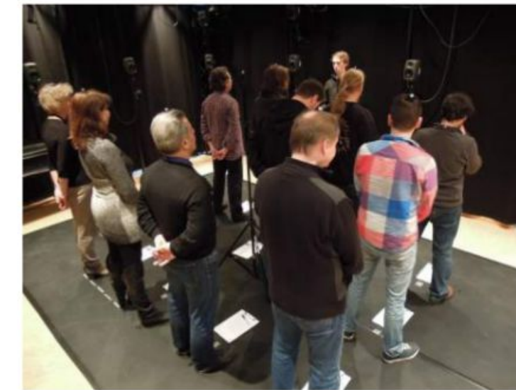
Figure 1. The setup for the "Norwegian Championship of Standstill." Each subject wore a reflective marker on the head, and one static marker was recorded from a standing pole in the middle of the space as a reference.
