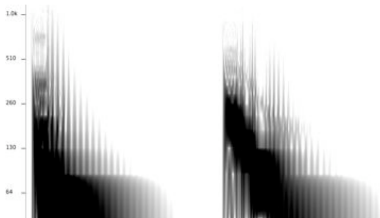
Figure 8.5: Sonograms of bass drum sounds from the Roland TR-808 to the left (tone: 3, decay: 3) and the TR-909 to the right (tone: 10, attack: 0, decay: 7).
