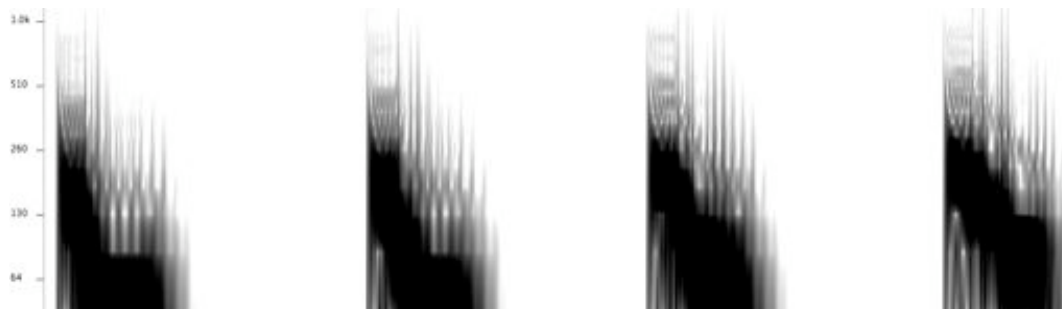
Figure 8.3: Sonogram of bass drum sounds from the Roland TR-909. Tune-settings, from left to right: 0, 3, 7 and 10 (attack: 0, decay: 0).
