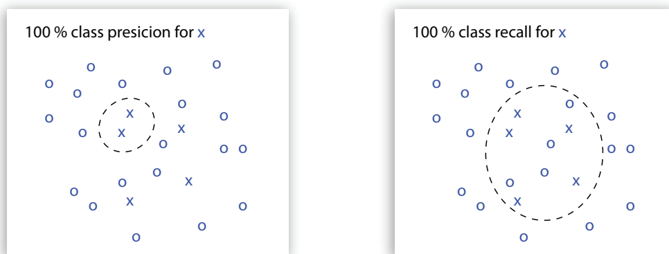
Figure 4.17: In the figure to the left 100 % class precision is obtained. However, several examples that should have been included are left out. To the right all the examples have been included in the classification. However, a number of incorrect examples are also included.
