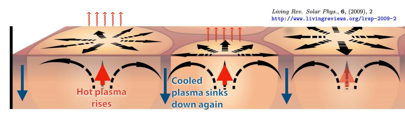
**Top of convection zone** — energy transport via convection (bulk motion)
