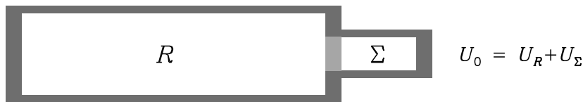
Figure 7.4: Simple system in thermal contact with reservoir
