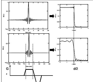
The effect of truncating the RF-excitation pulse (sinc-pulse). A 'perfect' slice profile requires an 'infinite' pulse duration and the truncation gives rise to a non-ideal slice profile as shown in the figure
