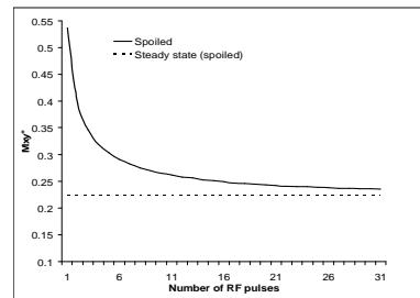
The progression of the  $M_{xy}$  (in relative units) towards a steady state level following multiple RF-pulses.
