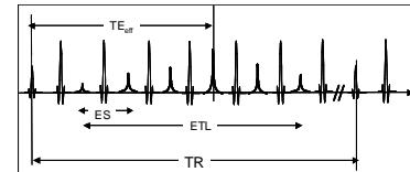
Signal (as fn of k-space line) is modulated by T2-relaxation with point-spread function given by:
