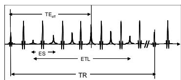
Signal (as fn of k-space line) is modulated by T2-relaxation with point-spread function given by:
