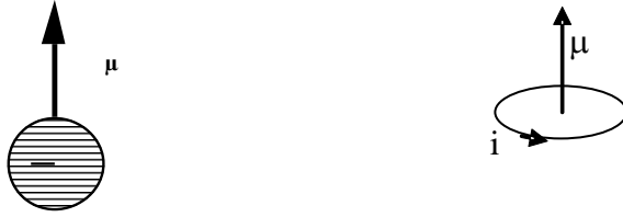
Figure 1. 4. A nuclear magnetic dipolemoment \mu , as formed by a combination of the internal spin and the the charge of the nucleus which results in a current i .
