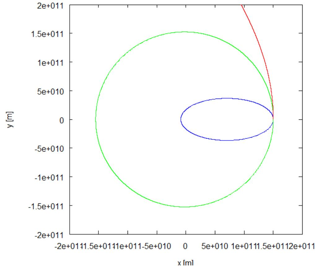
$$\begin{aligned}\vec{r}_0 &= x_0 \hat{i} \\ x_0 &= 1.5 \cdot 10^{11} \text{ m} \\ \vec{v}_0 &= v_0 \hat{j} \\ v_0 &= 1.0 \cdot 10^4 \text{ m/s} \\ v_0 &= 3.0 \cdot 10^4 \text{ m/s} \\ v_0 &= 4.5 \cdot 10^4 \text{ m/s}\end{aligned}$$
