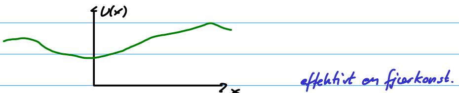
For små  $|x|$ :  $m\ddot{x} = -\frac{dU}{dx} = U'(0) + \underbrace{U''(0)x}_{\text{harm. osc.}} \Rightarrow \text{harm. osc.}$
