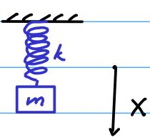
$$mg - kx = m\ddot{x}. \quad \text{Lihverkkt (i ro): } mg = kx_0 \Rightarrow x_0 = \frac{mg}{k}$$
