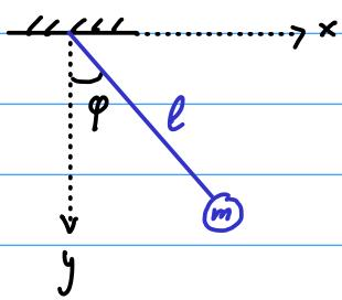
$$\text{Lagrange: } \frac{\partial L}{\partial \dot{\varphi}} = \frac{d}{dt} \left( \frac{\partial L}{\partial \dot{\varphi}} \right)$$
