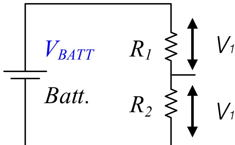
$$V_1 = \frac{R_1}{R_1 + R_2} V_{Batt}$$
