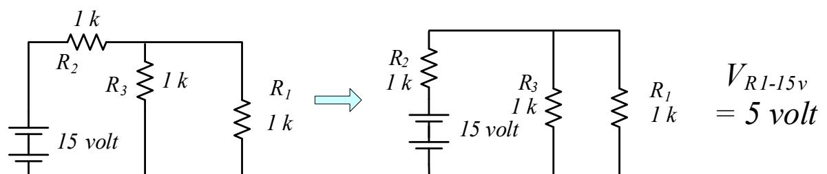
$$V_{R1} = 1 \text{ v} + 5 \text{ v} = 6 \text{ volt}$$
