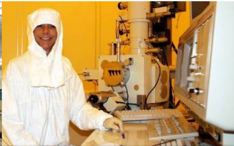
Scanning electron microscope for e-beam lithography
