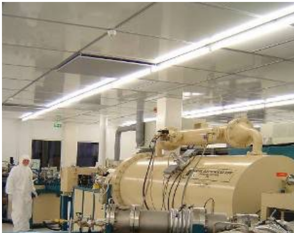
MeV ion accelerator 1 MVolt terminal voltage
