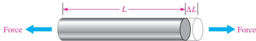
(a) Strain occurs as length changes from L to L + \Delta L when force is applied.
