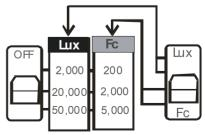
Example: If a measurement on the 5000 Fc range displays 350, then the actual measured value is; 350 X 10 = 3500 Fc.
