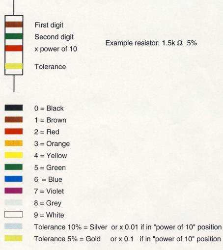
Five or six band resistors (metal film)
