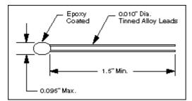
The ACCU-CURVE<sup>™</sup> device can also be supplied with 30 AWG solid Teflon insulated leads of 3, 6, 9 and 12 inches in length. contact RTI applications engineering for additional information.
