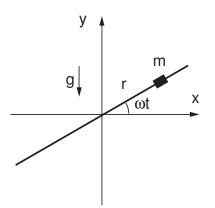
a) Find the Lagrangian for this system, expressed in terms of r,  $\dot{r}$  and t. Derive the corresponding Lagrange's equation.
