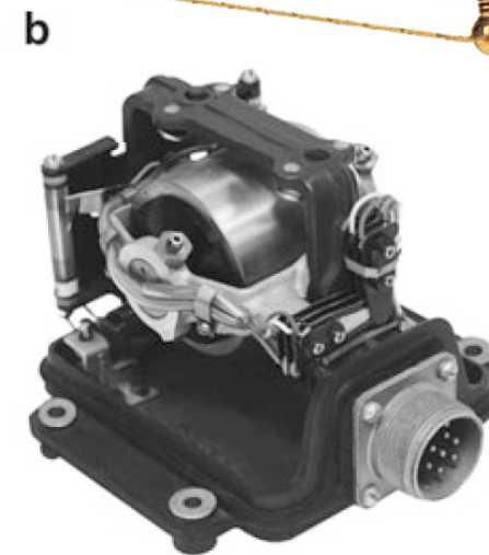
Fig. 8.10 Mechanical gyroscope with a single degree-of-freedom (a) and early auto-pilot gyroscope (b)
