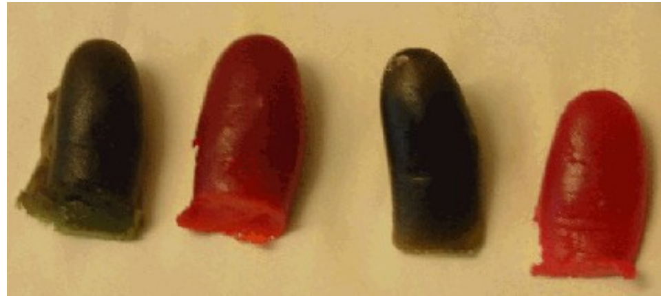
Index "gummy fingers" made from Matsumoto et al.'s recipe
