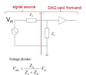
From the voltage divider equation we can se that we need to make sure that the DAQ device has a much higher input impedance  $Z_L$  than the signal source impedance  $Z_S$ , in order to get Vout  $\approx$  Vin.
