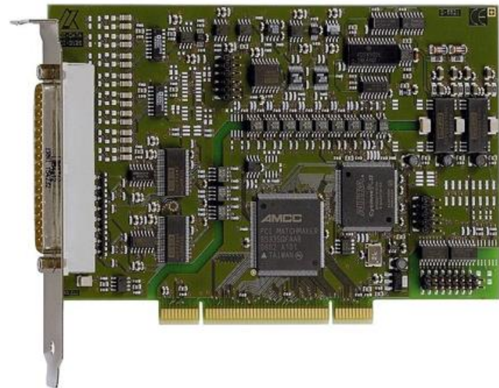
Figure 7-42. PCI interface card (ADDI-DATA APCI-3001)
