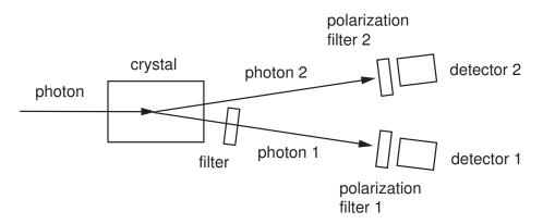
We assume in the following that a filter close to the crystal will single out photons only in the directions 1 and 2. This is schematically shown in Fig. 3. To analyze correlations between the two photons in each pair, polarization filters are applied to photons in both directions as also shown in the figure. Those that pass the polarization filters are registered in the detectors and the registrations are paired by use of coincidence counters.
