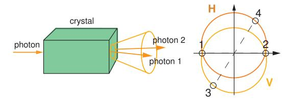
As a specific way to produce entangled photon pairs we consider the method of *parametric down conversion*, as described below and sketched in the Figure 2 and 3.
