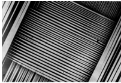
Fig. 11.11 Martensite. A particularly nice example of a martensitic structure, from Chu [30]. The light and dark stripes represent two different martensitic variants—that is, the crystal going through the phase transition can stretch in different directions, and the two colors indicate that the local lattice is stretching along two different axes. The tilted square region occupying most of the photograph could not change its overall shape without putting incompatible strains on the neighboring domains. By making this striped pattern, or laminar , the martensite can form an average of the different stretching directions that gives zero net strain.
