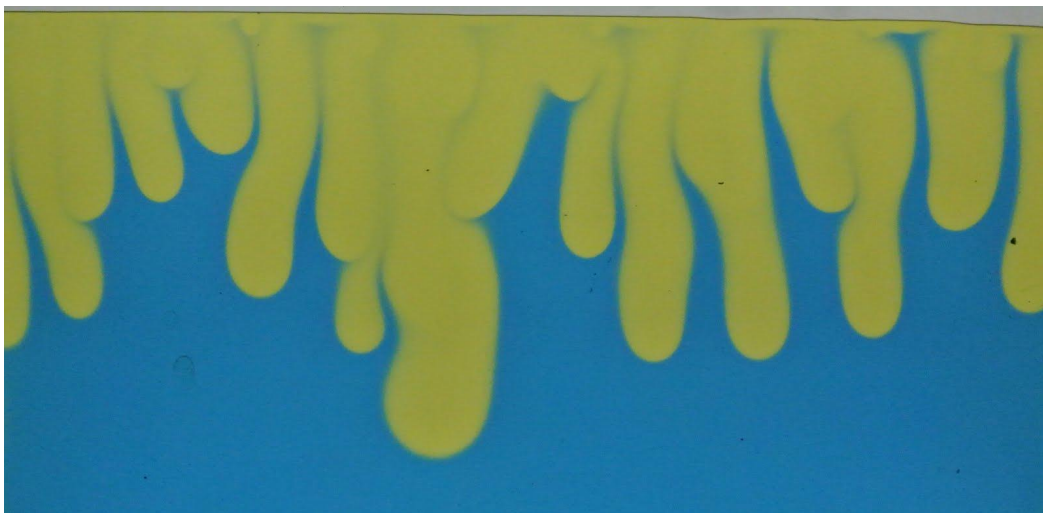
Figure 1: Visualisation of density-driven convection in a 2D system. The experimental setup simply consists of two vertical glass plates separated by a narrow gap. This system is initially filled with pure water mixed with a pH indicator giving a blue color. CO 2 is injected above the water level, and dissolves into the water, making the pH indicator turn yellow. Due to buoyancy, denser, CO 2 -rich water sinks, while less dense, pure water rises and convective fingers appear.
