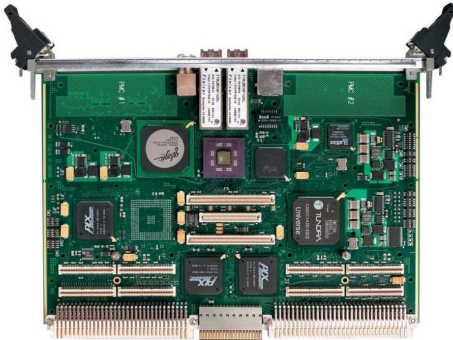
Figure 1 The MIDAS M5000 – VME version. Two PMCs can be mounted on the 2x4 PCI connectors.
