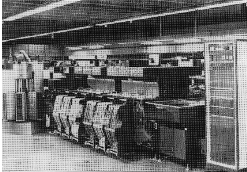
Fig. 7.36: Philips large hardware controlled pick-and-place machine.
