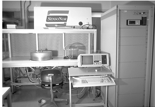
Fig. 9.13: The SensoNor/SINTEF Anodic Bonder. This equipment has a computer controlled bonding chuck for silicon wafers, facilitating flexible set up of bonding temperature and bonding voltage versus time with ramping. The equipment is built inside a flow box to avoid particle contamination. (Photograph courtesy of SensoNor, Horten, Norway)
