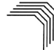
Typical Rigid Circuit Board Trace Routing
