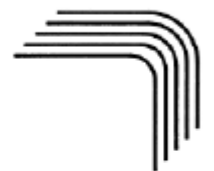
Typical Flexible Circuit Board Trace Routing
