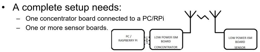
Only difference between the concentrator board and the sensor board are the code uploaded to the MCU, you shall only make on design!
