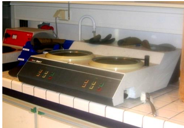
Grinding (thinning down to \sim 200 \mu\text{m} )
