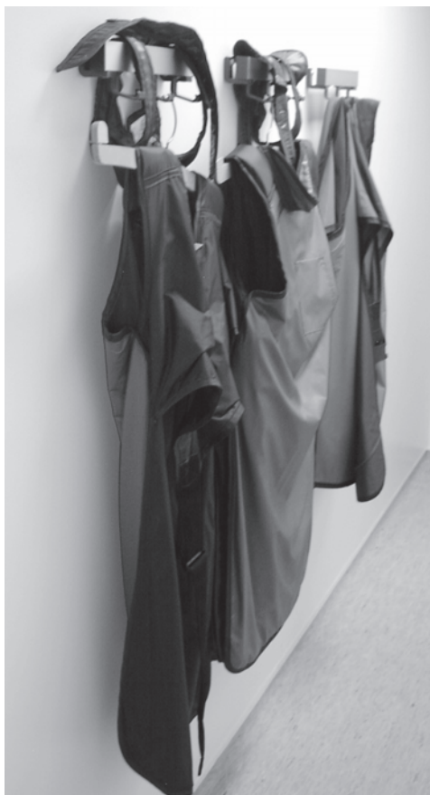
Figure 4.10 Lead aprons are suitable for reducing the effective dose to the body from diagnostic X-ray and low-energy photon sources only, but generally inadequate for most higher energy brachytherapy sources. With those sources the time of exposure during care-giving may be increased because of the apron, possibly leading to an even higher dose.
