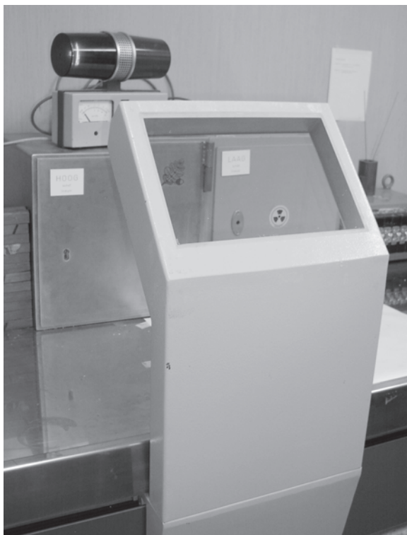
Figure 4.4 Details of a preparation table in a storage room, with a movable lead screen (5 cm Pb) with lead glass (9 cm thickness), and two vaults for storing different radionuclides.
