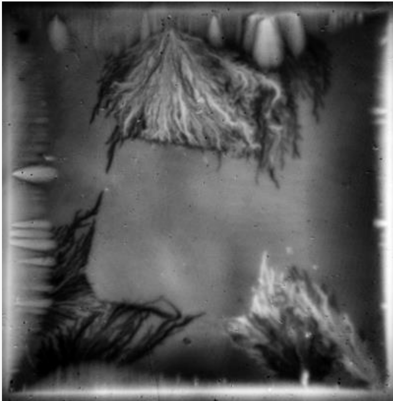
Distribution of magnetic flux in NbN superconducting film at 4 K.
