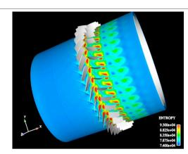
Calculation from the Stanford Center for Turbulence Research of a portion of the main compressor turbine in a modern jet engine. There are inflow and outflow boundaries as well as internal reflective boundaries for the turbine fan blades. The coordinate system rotates with the turbine, which starts slowly and approaches cruising speed.
