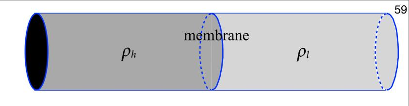
A closed tube filled with gas, separated by a membrane into sections with different densities.
