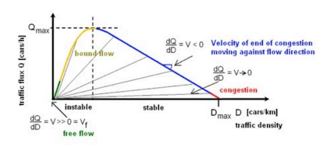
V<sub>f</sub> = "free velocity" - maximum velocity on free lane, selectable by the driver depending on car, skill etc.
