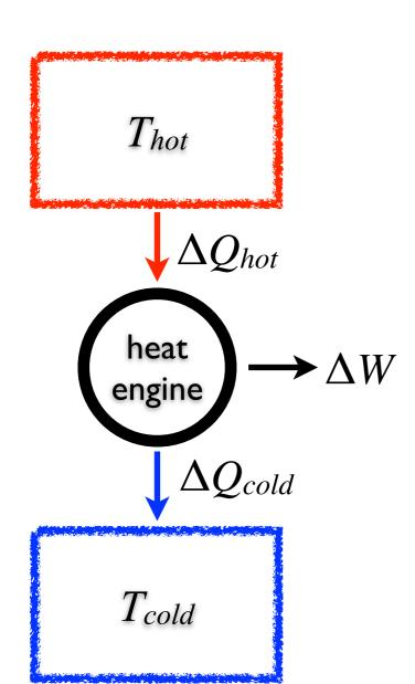
$$\Delta W_{\text{reversible}} = \Delta Q_{\text{hot}} - \Delta Q_{\text{cold}}$$
